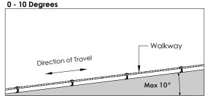
Roof Angle: 7° - 10° - Walkway same angle as roof
