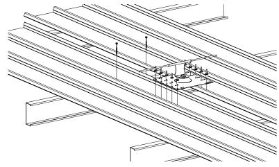
Details for 3 - 9 purlins 2 x 14G Fixings into purlin above OR below anchor plate
